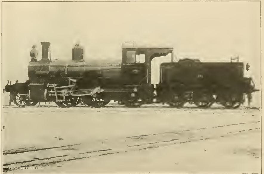
TWO CYLINDER COMPOUND MOGUL, NORWEGIAN STATE RAILWAYS. WITH WALSCHAERT VALVE MOTION.
